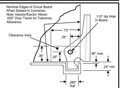
Detail View of Actuating Surface and Circuit Board Shown for Reference Only
