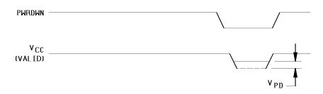
NOTE: All timings except  $t_{TSHZ}$  and  $t_{TSON}$  are measured at 1.5 V levels with 50 pF minimum output load. For input signals, rise and fall times are less than 6.0 ns, with low amplitude = 0 V, and high amplitude = 3.0 V.
