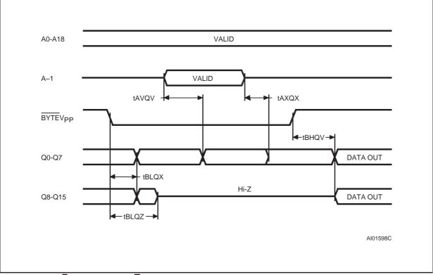
Note: Chip Enable ( $\overline{E}$ ) and Output Enable ( $\overline{G}$ ) = V<sub>IL</sub>.
