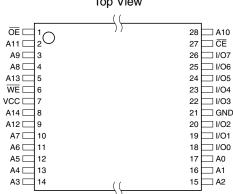
PDIP, SOIC Top View
