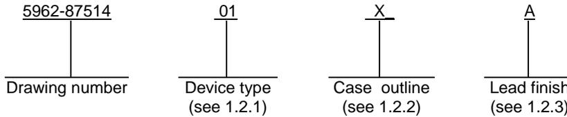
1.2.1 Device type(s). The device type(s) shall identify the circuit function as follows:
