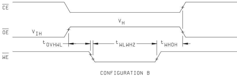
FIGURE 8. Chip clear waveforms.
