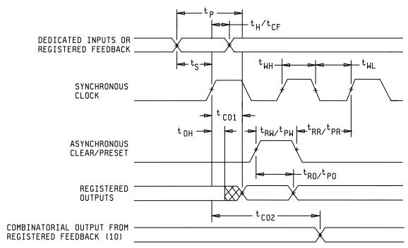
FIGURE 4. Switching waveforms.
