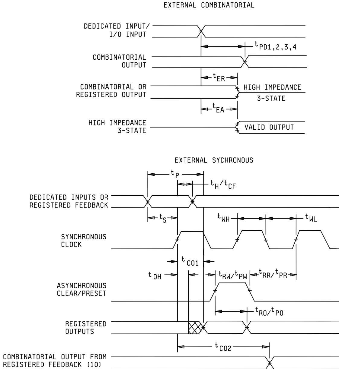
FIGURE 4. Switching waveforms.
