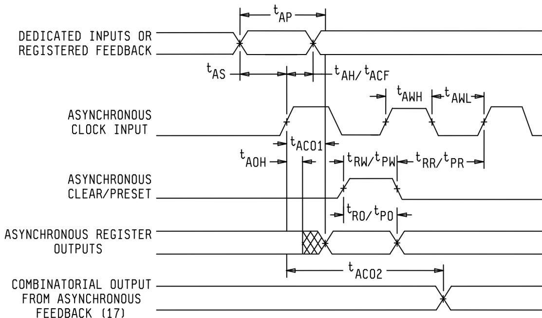
FIGURE 4. Switching waveforms - Continued.
