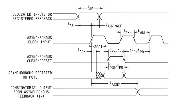
FIGURE 4. Switching waveforms - Continued.
