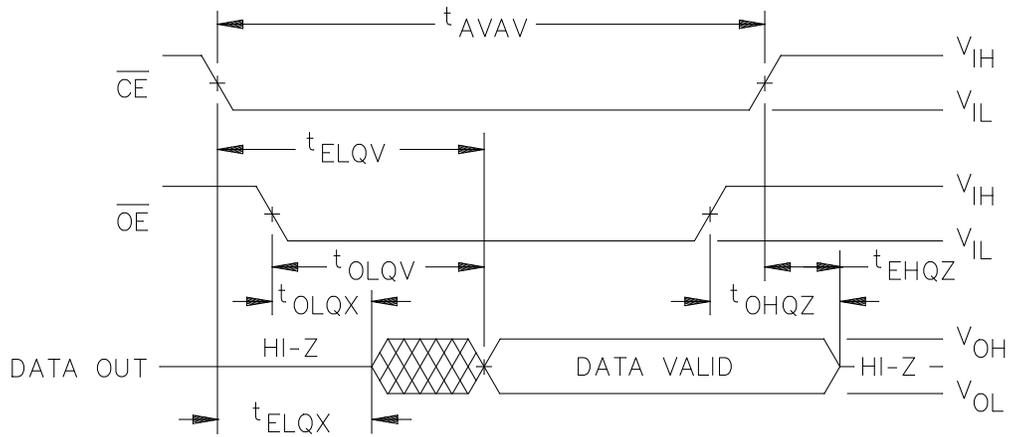
NOTE: When  $\overline{WE}$  is high, address is valid prior to or simultaneously with the high to low transition of  $\overline{CE}$ .
