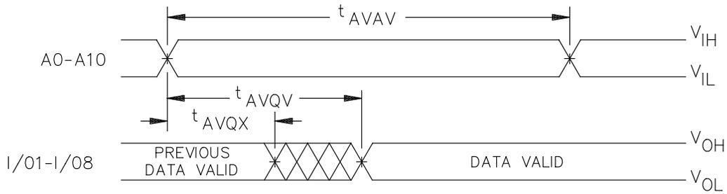
NOTE: When  $\overline{WE}$  is high, address is valid prior to or simultaneously with the high-to-low transition of  $\overline{CE}$ .
