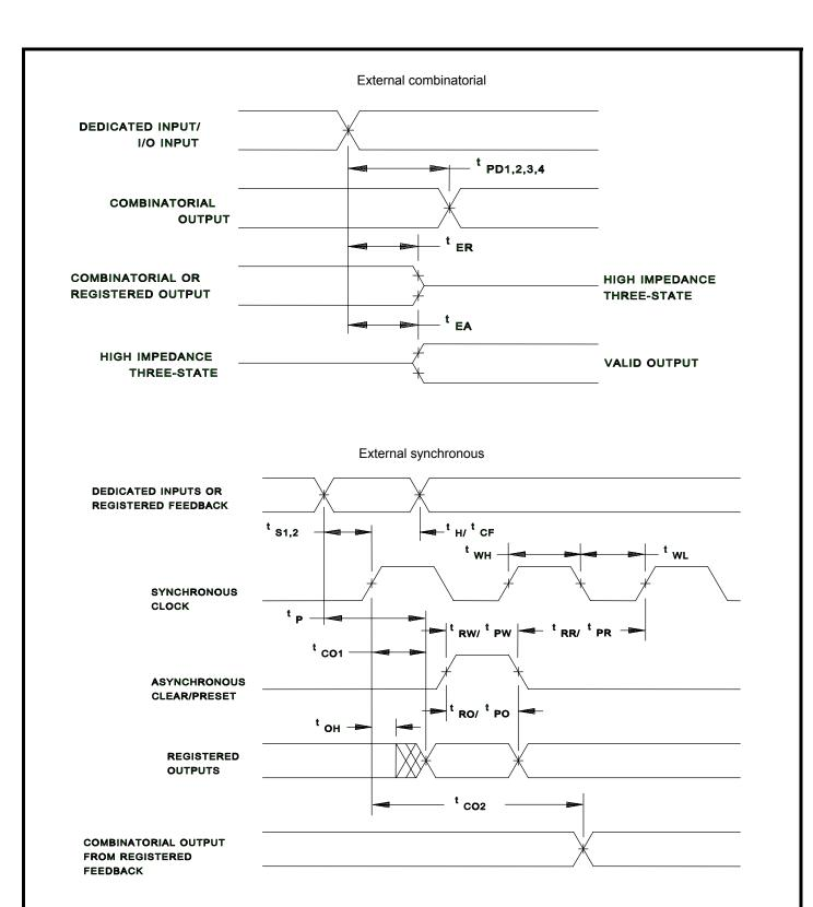
FIGURE 4. Switching waveforms.
