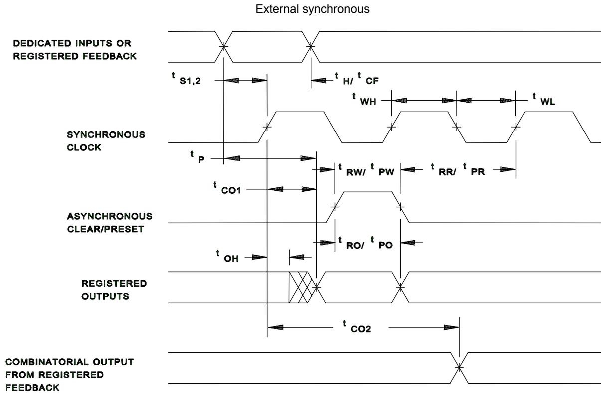
FIGURE 4. Switching waveforms.
