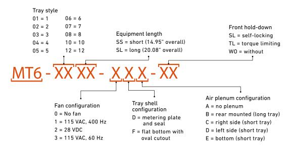
Contact us if fan or shock vibration isolators are required. We will generate a part number based on the configuration you select.
